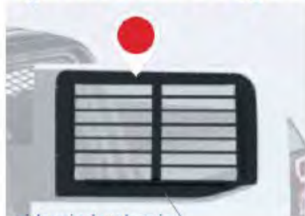
side window barrier
