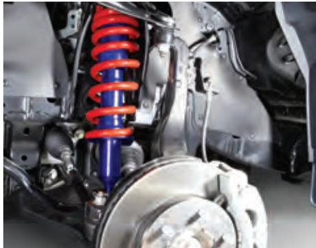
Upgraded brake and suspension package
