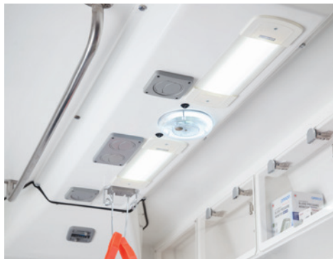
Cabin ceiling services panel
